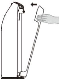
Carefully install front plate as shown on the left.
