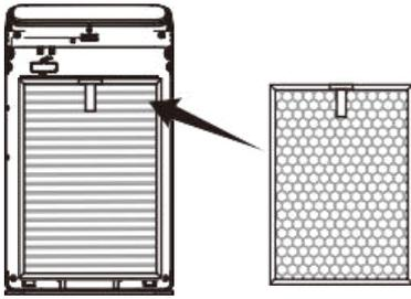
Install filter 2 (activated carbon & cold catalyst compound filter)
