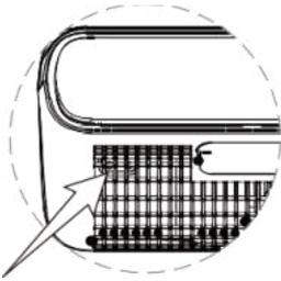
3. Clean the ionizer by carefully inserting a soft, clean brush pen into the holes of the grille. Do only exert low pressure while cleaning.
