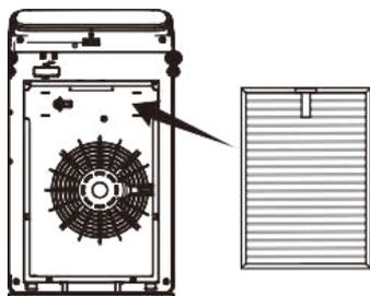
Install filter 3 (HEPA-13 & antibacterial compound filter)
