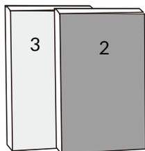
2 Activated carbon & cold catalyst compound filter
