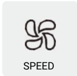
The speed control can be set to low (500 RPM), medium (700 RPM) or high (900 RPM). The current speed is shown on the digital screen. When pressing the button while the highest level is active, the speed will switch to lowest level again.
