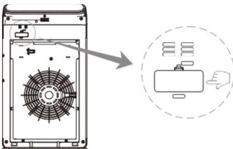
4. Now use a dry cotton swab to clean the exposed particle sensor area.
