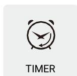
Press this button to set the working time. Every push increases the working time by 30 minutes. You can set between 1 - 12 hours and the device is turned off when the timer expires.
