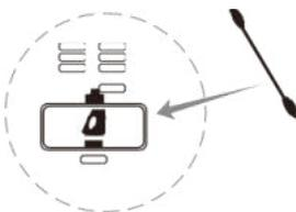
5. When finished, put the particle sensor cover back to its original position and close the front plate as shown in the chapter *Installation*.
