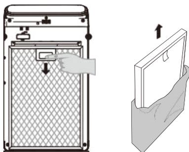
Take out the filters by pulling on the respective strip and remove all packaging bags from the filters.
